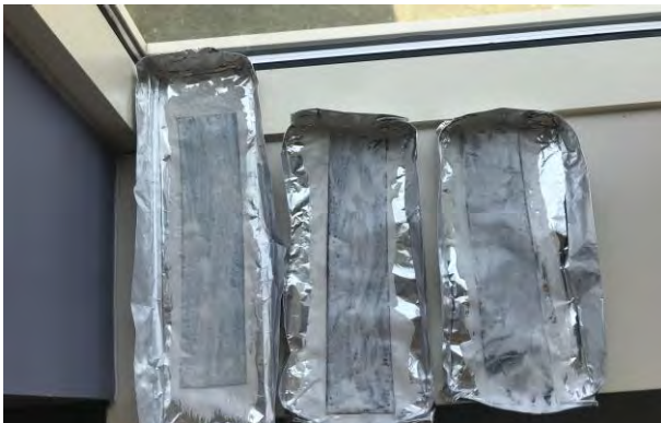
Figure 5. Thin-layers of paper-mache applied to the graphene-painted strips.
